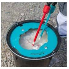
Place the dirty mixing paddle between the brushes, make the mixer rotate slowly until it is completely immersed. In order to guarantee that the mixer is cleaned properly, hold it in a slightly inclined position while it is rotating.
