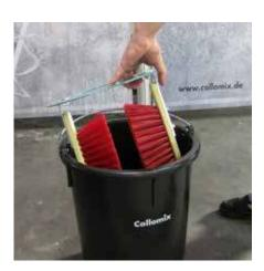
After the cover with the brushes has been taken out, the water and dirt at the bottom can be poured out.
