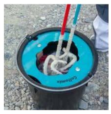
After mixing, clean the mixing paddle from material freshly stuck to it with the help of Mixer-Clean.
